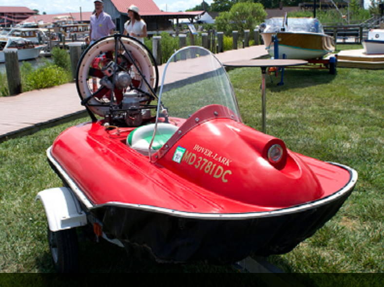
1967 Hoverlark Hovercraft Manufactured by Hover-Air of Peterborough 1967-1971 One of the smallest Hovercraft designed to ride on the roof of a car. Top Speed 45 MPH on Water 25 Mph on land Presented in 1990 to the Chesapeake Bay museum by Rev. Granville
